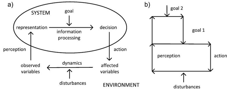
Figure 1: (a) Model of a control system. (b) Double loop control system (Source [4]).
